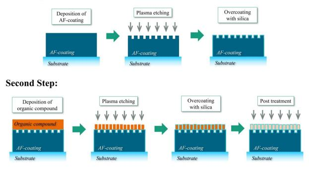
To make the multifunctional coating system, the researchers applied a technology that allows several nanostructures to be created on top of each other. The process involved etching a nanostructure into the antifog coating and then fabricating a second nanostructure on top. Credit: Anne Gärtner, Fraunhofer Institute for Applied Optics and Precision Engineering and Friedrich Schiller University Jena
