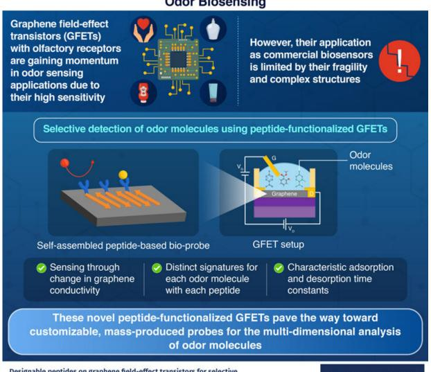
Designable peptides on graphene field-effect transistors for selective detection of odor molecules
