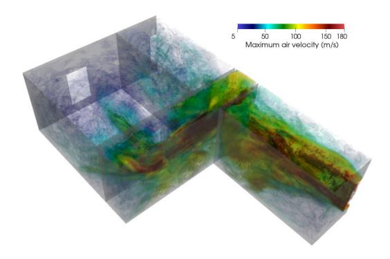
Contours of the maximum airspeed attained during the first 10 seconds after the blast wave enters the window; overpressure of 5 psi. Credit: I. Kokkinakis and D. Drikakis, University of Nicosia, Cyprus
