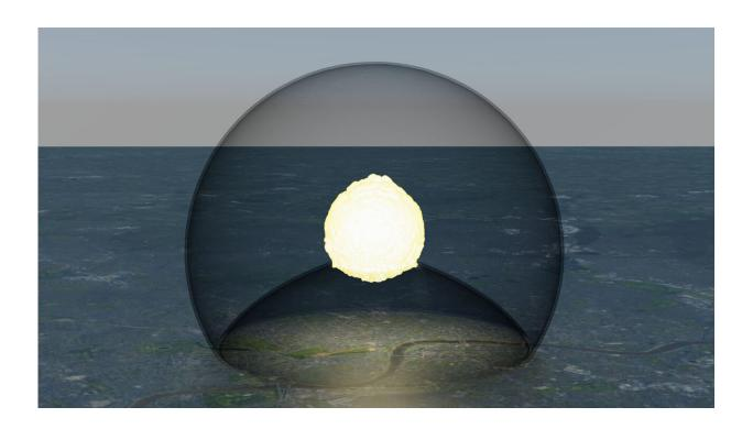
3D illustration of the simulated air blast and generated blast wave 10 seconds following the detonation of a 750 kT nuclear warhead above a typical metropolitan city; the radius of the shock bubble at ground level is 4.6 km. Credit: I. Kokkinakis and D. Drikakis, University of Nicosia, Cyprus
