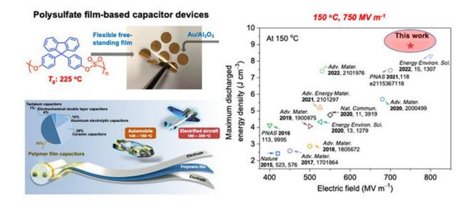
Polysulfates with excellent thermal properties are casted into flexible freestanding films. High-temperature, high-voltage capacitors based on such films show state-of-the-art energy storage properties at 150 degrees C. Such power capacitors are promising for improving the energy efficiency and reliability of integrated power systems in demanding applications such as electrified transportation by mass and volume reductions. Credit: Scripps Research
