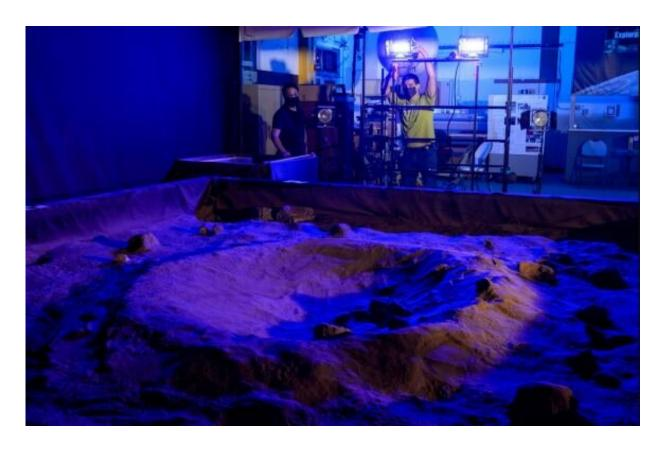
In the Regolith Testbeds at NASA's Ames Research Center, which are designed to mimic lunar terrain as it would appear in different areas at the Moon's poles, the VIPER team tests out lighting systems for the rover with a very low-angle illumination simulating the Sun. Credit: NASA/Dominic Hart
