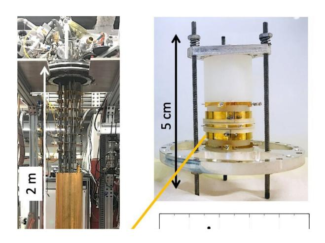
(Left) dilution refrigerator used to achieve background-free single electron quantum cyclotron. (Top right) silver Penning trap inside which the single electron will be suspended. (Bottom right) demonstration of resolution of quantum cyclotron states. A microwave drive is applied to induce the transition. Credit: Xing Fan.
