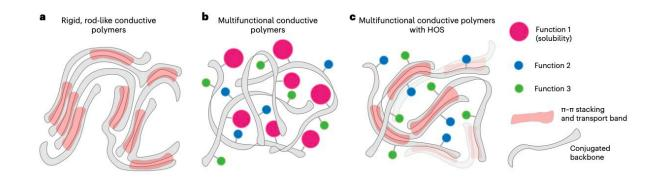
Proposed chemical and morphological evolution of conductive polymers. a–c, Schematic illustration of polymer chain arrangements in rigid, rod-like conductive polymers (a); multifunctional conductive polymers (b) and multifunctional conductive polymers with HOS (c). Credit: Zhu et al. (*Nature Energy*, 2023).
