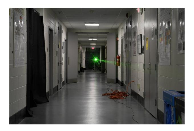
A laser is sent down a UMD hallway in an experiment to corral light as it makes a 45-meter journey. Credit: Intense Laser-Matter Interactions Lab, UMD
