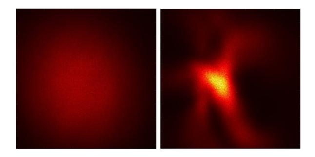
Distributions of the laser light collected after the hallway journey without a waveguide (left) and with a waveguide (right). Credit: Intense Laser-Matter Interactions Lab, UMD
