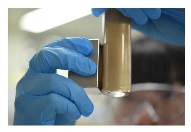
Researchers at UQ's Australian Institute for Bioengineering and Nanotechnology have developed a way to remove PFAS chemicals from water using a magnet. Credit: University of Queensland
