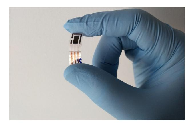
Flexible copper sensor made cheaply from ordinary materials: conductive copper adhesive tape, sheet of transparency film, paper label, nail varnish, circuit fabrication solution, and acetone. Credit: Anderson M. de Campos
