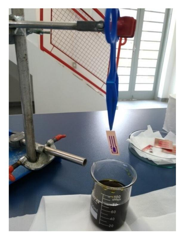
The sensor's lead and cadmium detection performance was validated in trials using artificial sweat. Credit: Anderson M. de Campos
