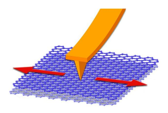
Schematic illustration of the atomic force microscopy-based (AFM) nanoscale friction test setup. A silicon AFM probe (covered with native oxide) slides on the graphite (0001) basal plane. The normal load between the silicon tip and the graphite surface is applied via bending the cantilever. While the probe is moving along the red arrows, the cantilever twists due to the friction force at the contact point between the silicon tip and the graphite surface. The degree of the twisting
