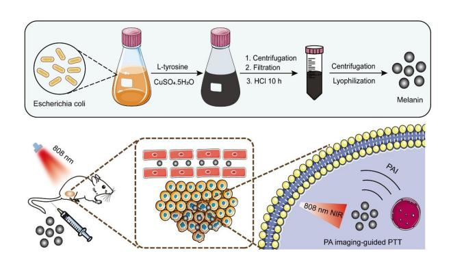
Schematic illustration of biosynthetic melanin nanoparticles for photoacoustic imaging-guided photothermal therapy. Credit: SIAT
