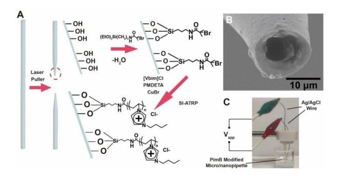
Fabrication of PFM. (A) Preparation of PFM with laser puller and SI-ATRP. (B) SEM image of the 10-µm-diameter tip of a PFM. (C) Experimental setup for the electric measurement with the PFM. Credit: *Science* (2023). DOI: 10.1126/science.adc9150
