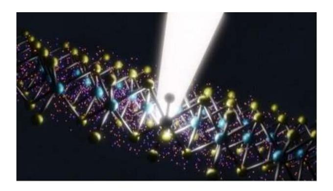
Stanford scientists are revealing the virtual quantum states formed in novel twodimensional materials subjected to intense laser pulses. In the experiments, midinfrared laser beam is focused to monolayers of tungsten disulfide, where the strong electric field of the laser interacts with excitons—electron-hole pairs therein. Credit: Yuki Kobayashi.
