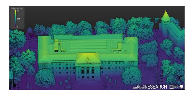
This image of the Neue Universität at Sanderring was generated from elevation data. The different colours indicate the distance to the ground. Credit: Chair of Remote Sensing / University of Würzburg
