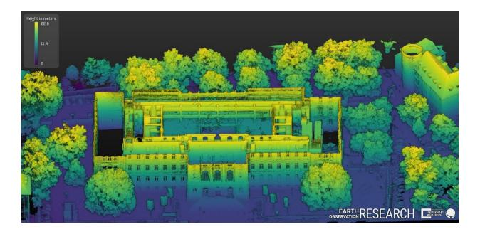
Deriving an elevation of the university building at Sanderring is also possible by combining airborne and ground-based lidar systems. Credit: Chair of Remote Sensing / University of Würzburg
