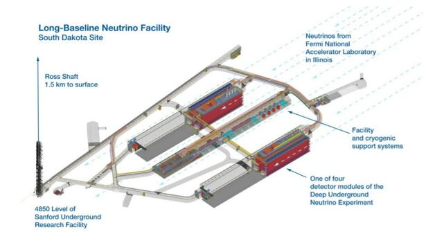
Almost 800,000 tons of rock need to be excavated to create the space for the South Dakota portion of the Deep Underground Neutrino Experiment. Half of the excavation is now complete. Credit: Fermilab
