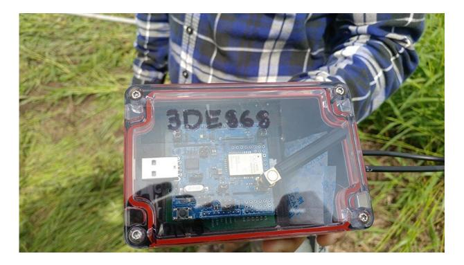
The network's communication nodes (above) are encapsulated in clear, waterproof plastic and buried a foot and a half below the surface. Credit: Guha Lab
