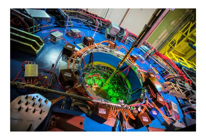
The house-size STAR detector at the Relativistic Heavy Ion Collider (RHIC) acts like a giant 3D digital camera to track particles emerging from particle collisions at the center of the detector. Credit: Brookhaven National Laboratory
