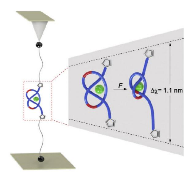
Depiction of the interfacing of the molecular knot between the AFM tip and the substrate. The knot (in blue) conformation is maintained by coordination to a Lu<sup>3+</sup> ion (in green). Two poly(ethylene glycol) chains are used as tethers for the trapping of the knot between the tip and the substrate. The mechanical tightening of the knot is associated with an incremental distance of 1.1 nm. Credit:
