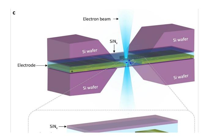
Schematic illustration of the electrochemical liquid cell. Credit: Yang, R. et al. https://www.nature.com/articles/s41596-022-00762-y
