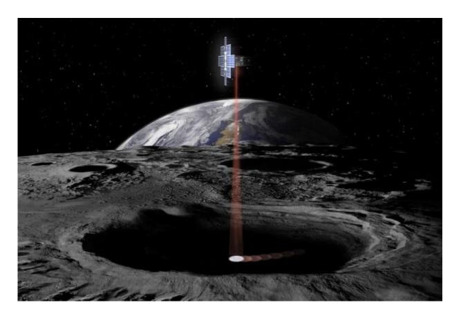
Finding and extracting oxygen from lunar ice will involve different missions as part of the effort. In this artist's illustration, NASA's Lunar Flashlight's lasers are scanning a shaded lunar crater for the presence of ice. Credit: NASA/JPL-Caltech
