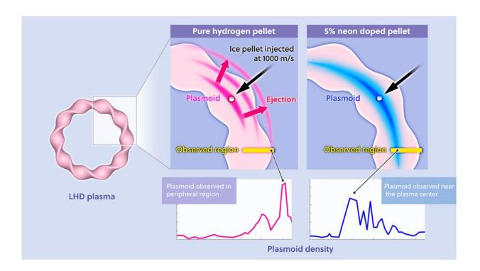
Plasmoid behavior of pure hydrogen and hydrogen mixed with 5 % neon. In this experiment, a new Thomson Scattering (TS) diagnostic system operating at (an unprecedented rate of) 20 kHz was used to (i) measure the density of the plasmoid at the moment it passed through the observation region, and (ii) identify its position, which verified the theoretical predictions. Credit: National Institute for Fusion Science
