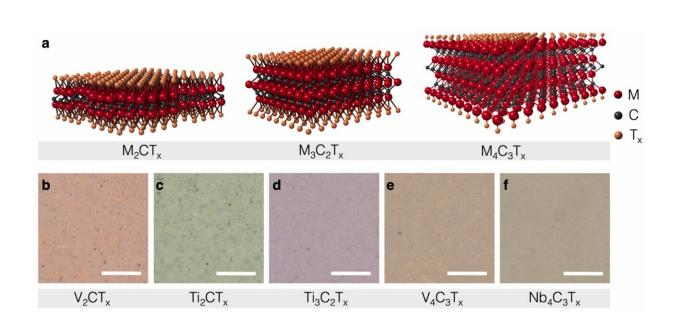
MXene electrodes used in this work. a, Schematics of MXene with different numbers of atomic layers. Optical images of (b)  $V_2CT_x$ , (c)  $Ti_2CT_x$ , (d)  $Ti_3C_2T_x$ , (e)  $V_4C_3T_x$ , and (f)  $Nb_4C_3T_x$ . Scale bar, 20 µm. Credit: *Nature Nanotechnology* (2023). DOI: 10.1038/s41565-022-01308-9
