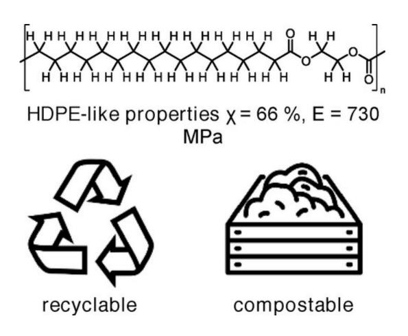
While it resembles high density polyethylene with regard to its mechanical properties and solid-state structure and has a high melting point (Tm=96 °C), the novel polyester-2,18 material at the same time fully hydrolyzes in in vitro enzymatic degradation studies and mineralizes under industrial composting conditions (ISO standard 14855-1) within two months. Credit: *Angewandte Chemie International Edition* (2022). DOI: 10.1002/anie.202213438
