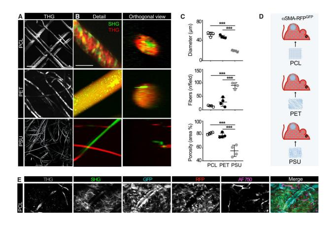
Longitudinal intravital imaging of the FBR in the three different biomaterials. (A) 3D reconstruction of PCL, PSU, and PET scaffolds by THG, macroscopic
