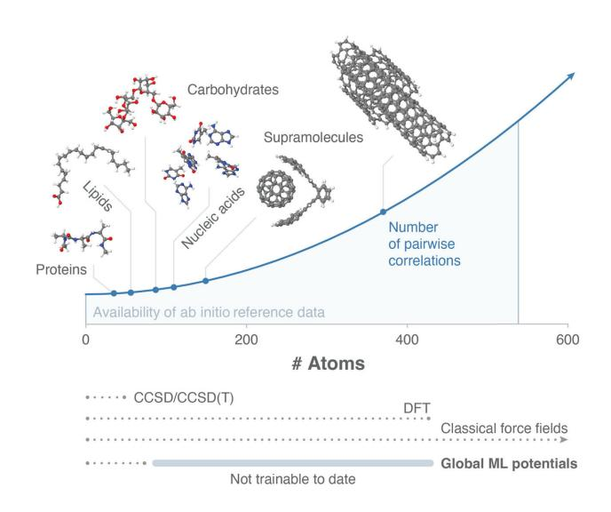
Current global MLFFs only scale to system sizes of a few dozen atoms, restricted by the computational challenge of having to couple a quadratic amount of atomatom interactions. However, accurate ab initio reference data are available for much bigger systems (light blue area). This work scales global models with ab
