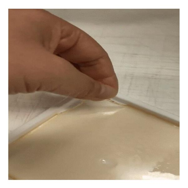
This image shows the soft and stretchable material for use in wearable sensors. Credit: Xiaohong Lan, University of Groningen
