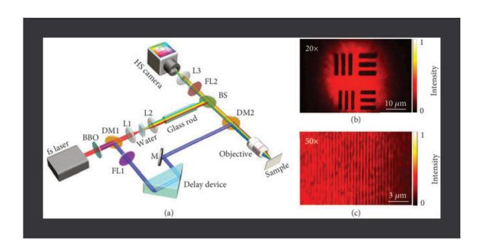
Configuration of CSMUP. (a) Experimental device of CSMUP. (b) Imaging a 1951 USAF resolution test target with a 20× objective. (c) Imaging a grating of 1200 lp/mm with a 50× objective. Credit: *Ultrafast Science* (2022). DOI: 10.34133/2022/9842716
