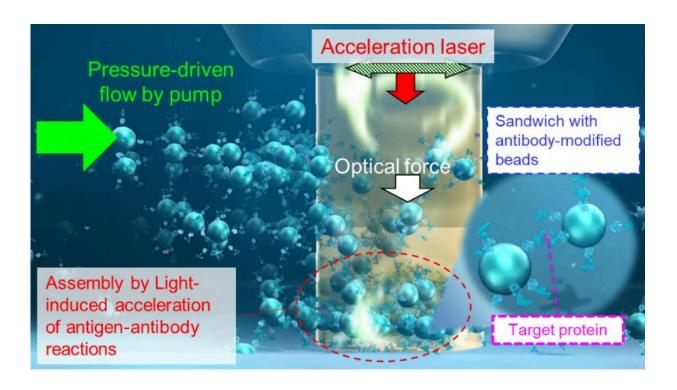
Illustration of the principle underlying the detection of trace amounts of proteins: Osaka Metropolitan University researchers introduced target proteins and probe particles with modified antibodies selectively binding to the target proteins into a small channel and applied irradiation with infrared laser light. They achieved, for the first time, the rapid measurement of trace amounts of attogram-level target proteins after only 3 minutes of laser irradiation. Credit: Takuya Iida, OMU
