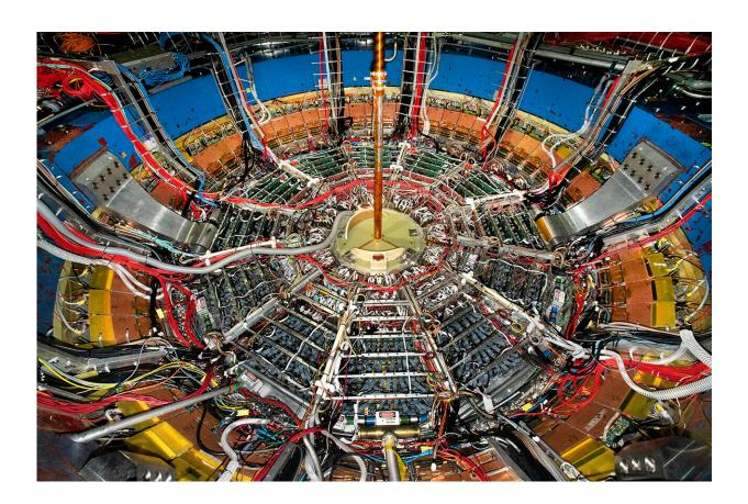
A comprehensive analysis of data from the STAR detector at the Relativistic Heavy Ion Collider (RHIC), above, reveals that conditions created just as heavy ions collide in the center of the detector have the biggest influence on the asymmetric flow of particles from these collisions. The results will help scientists zero in on key properties of a unique form of matter that mimics the early universe. Credit: Brookhaven National Laboratory
