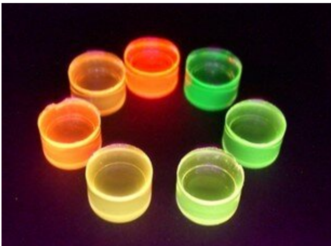
Figure 3: The molecular design method has the potential to create phosphors that emit different colored light when applied to different luminescent complexes. Credit: Toshiba Corporation News Releases
