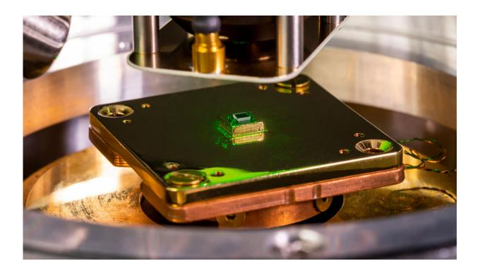
Using specially designed diamonds with nitrogen-vacancy centers, researchers at Princeton University and the University of Wisconsin-Madison have developed a technique to measure noise in a material by studying correlations, and they can use this information to learn the spatial structure and time-varying nature of the noise. In this image, a diamond with near-surface nitrogen-vacancy centers is illuminated by green laser light from a microscope objective lens. Credit: David Kelly Crow
