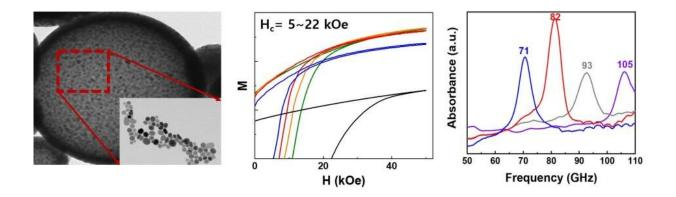
The shape, magnetic properties and electromagnetic wave absorption properties of the epsilon iron oxide. Credit: Korea Institute of Materials Science (KIMS)
