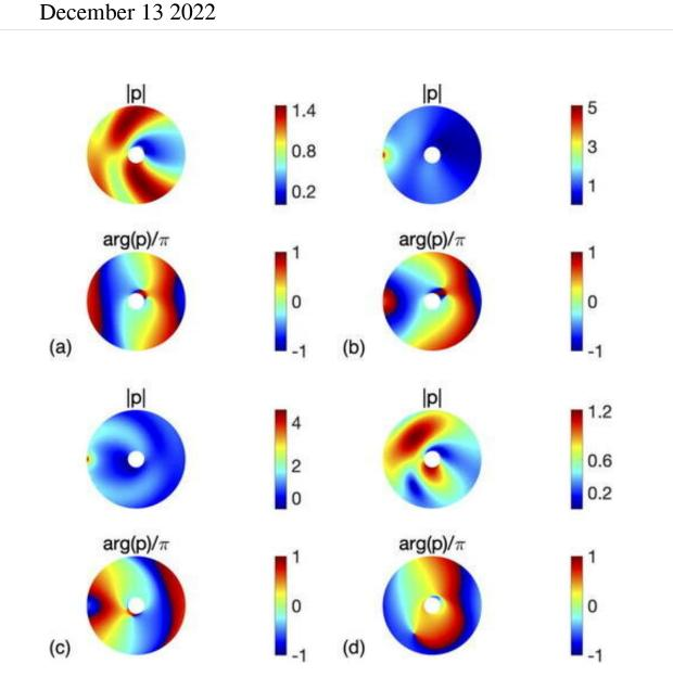
lpl and  $arg(p)/\pi$  of total pressure in the presence of a spinning cylinder with radius a = 0.35 m (white disks) and  $\rho = 1000 \text{ kg/m}^3$  and  $1/\beta = 2.22 \text{ GPa}$ , for
