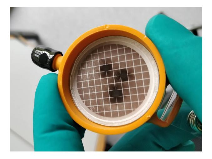
After testing, content of filters were analyzed. Especially iron particles showed up in high concentrations. Credit: Hugo Savill Russell
