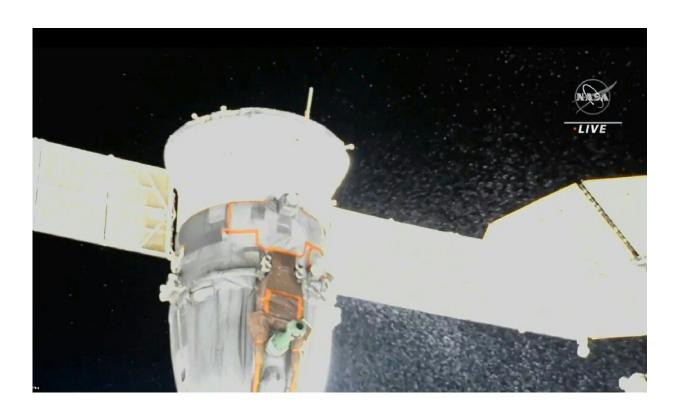
The vehicle, known as MS-22, began spraying its coolant into space on December 14, with dramatic NASA TV images showed white particles resembling snowflakes streaming out of the rear.
