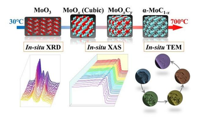
In situ investigations on structural evolutions during the facile synthesis of cubic  $\alpha$ -MoC<sub>1-x</sub> catalysts. Credit: Yu Jiafeng
