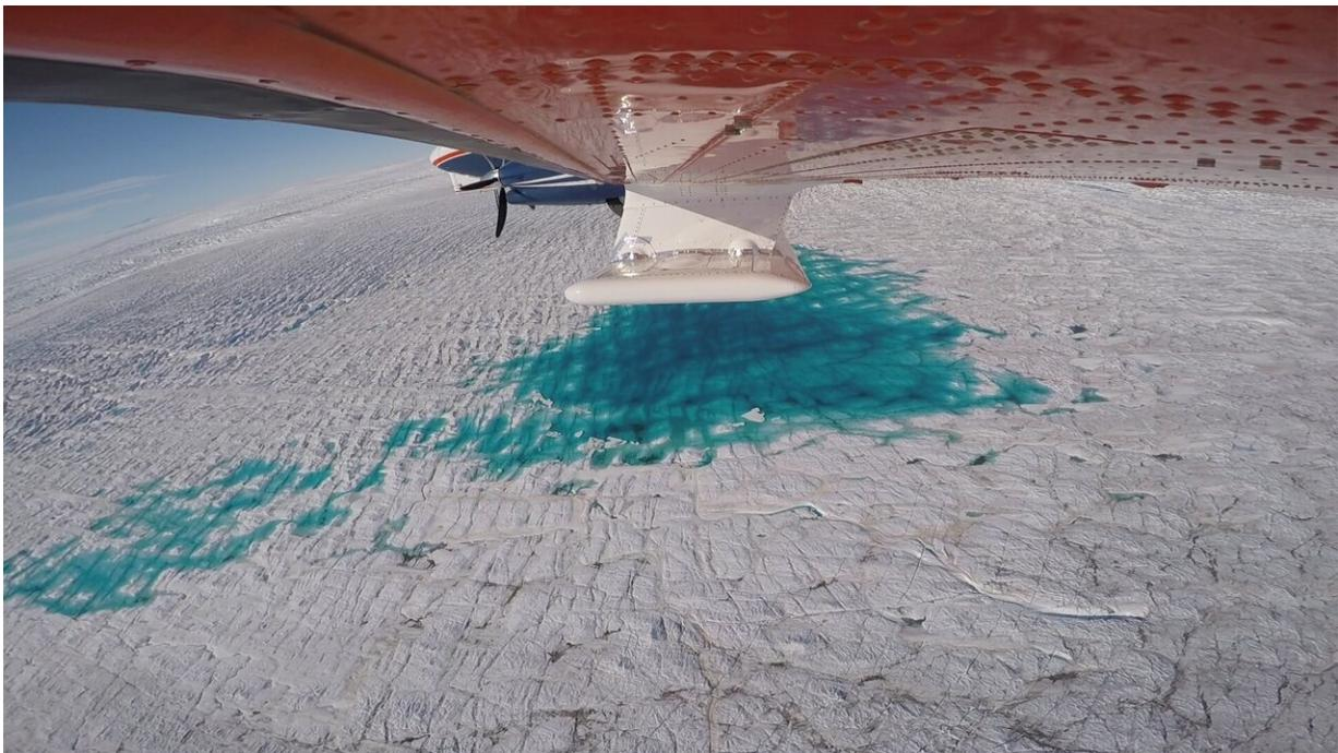
Measuring ice thickness with the ultra wideband ice radar system, attached to the aircraft's wings. Credit: Alfred-Wegener-Institut / Tobias Binder
