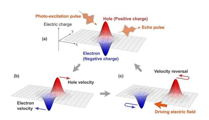
A schematic diagram of the present echo-generation process. (a) An electronhole pair is created by a photo-excitation pulse. (b) After the excitation, the electron and hole move in opposite directions. (c) A driving electric-field pulse reverses the relative velocity of the electron-hole pairs, resulting in the recombination of the pairs and the emission of echo pulses. Credit: Atsushi Ono
