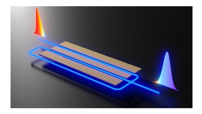
Changing the color of single photons using an integrated phase modulator. Credit: Loncar Lab/Harvard SEAS
