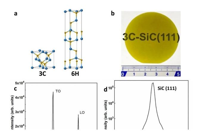
Structure of wafer-scale free-standing 3C-SiC bulk crystals. a Atomic structures of 3C-SiC and 6H-SiC. b Picture of a 3C-SiC 2-inch wafer. The unit of the ruler is cm. c Raman spectrum of 3C-SiC crystal. d X-ray diffraction (XRD) of 3C-SiC. e High-resolution STEM image of 3C-SiC taken along the [110] zone axis. The inset: Fast Fourier transform (FFT) of the STEM image. f Selected area electron diffraction pattern of 3C-SiC taken in the [110] zone axis. Credit:
