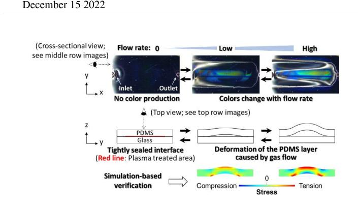
Mechanism behind the multi-color imaging of a gas injected into the device. Top (top row) and cross-sectional (middle and bottom rows) views of the device and a gas flowing through it. Credit: Kota ShibaNational Institute for Materials Science
