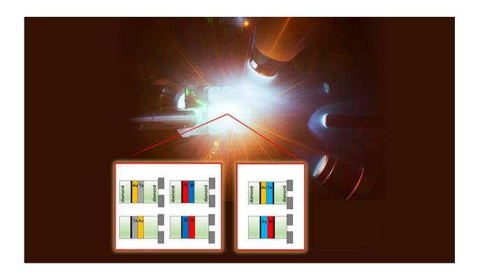
Optical photograph taken during a laser-driven compression and nanosecond Xray diffraction experiment at the Omega Laser Facility. The inset illustrates the specific target configuration used in this study, where multiple samples were simultaneously compressed along a quasi-isentropic path. Graphic credit: Kowaluk/LLE and Coppari/LLNL
