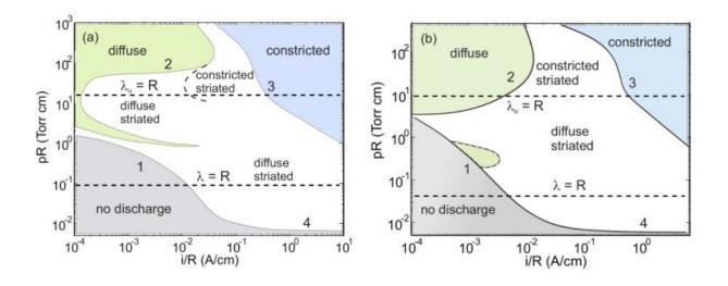
Discharge forms in Neon (a) and Argon (b) for different currents i and gas pressures p. Credit: *arXiv* (2022). DOI: 10.48550/arxiv.2208.14321
