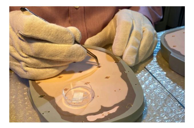
Installation of passive thermoluminescent detectors in the phantom. Credit: Source: DLR
