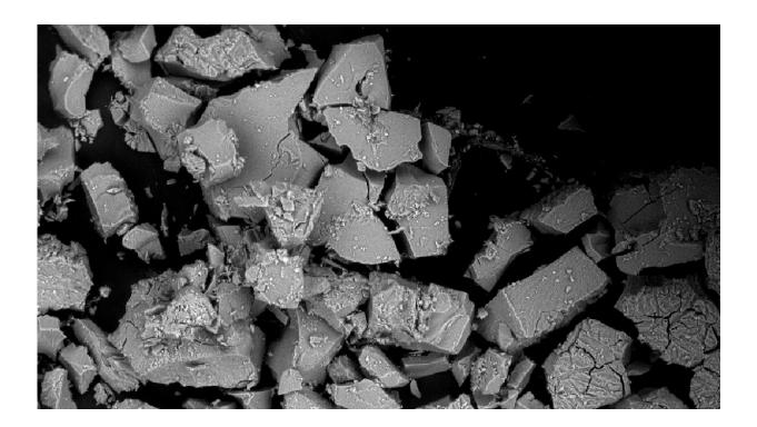
Scanning electron microscopy image showing a precipitated hydrated calcium carbonate mineral (Ikaite), which could be used for ocean alkalinity enhancement for carbon dioxide removal from the atmosphere. Credit: Dr Laura Bastianini (Heriot-Watt University)
