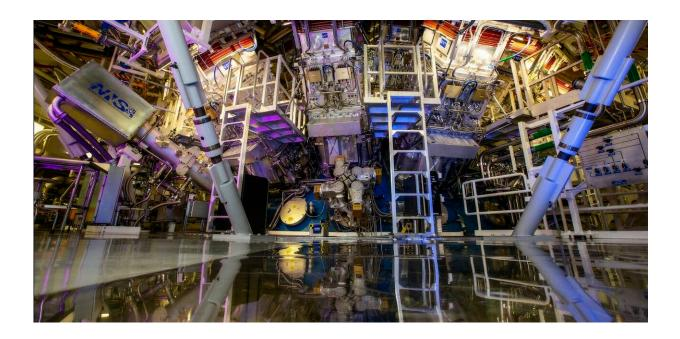
NIF's target chamber, where a powerful laser is used to start nuclear fusion reactions. Credit: Jason Laurea/Lawrence Livermore National Laboratory (LLNL), CC BY-NC-SA
