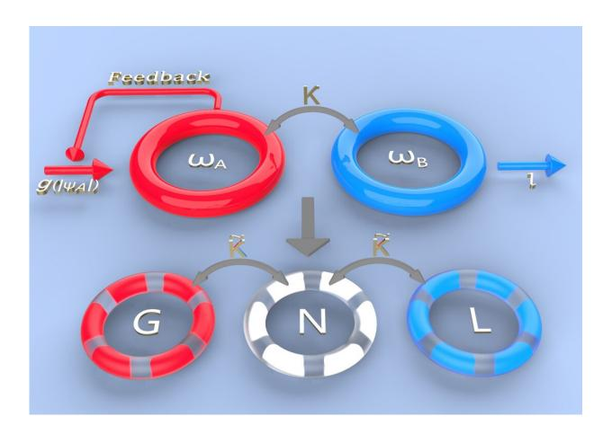
The upper panel shows two coupled resonators. The left resonator (red) has nonlinear saturable gain, and the other resonator (blue) has linear loss. Such a nonlinear non-Hermitian system can be mapped into a PT symmetric three-resonator system as shown in the lower panel with linear gain (G), neutral (N) and loss (L) resonators. Credit: Science China Press
