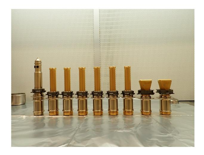
The drill bits used by NASA's Perseverance rover are seen before being installed prior to launch. From left, the regolith bit, six bits used for drilling rock cores, and two abrasion bits. Credit: NASA/JPL-Caltech
