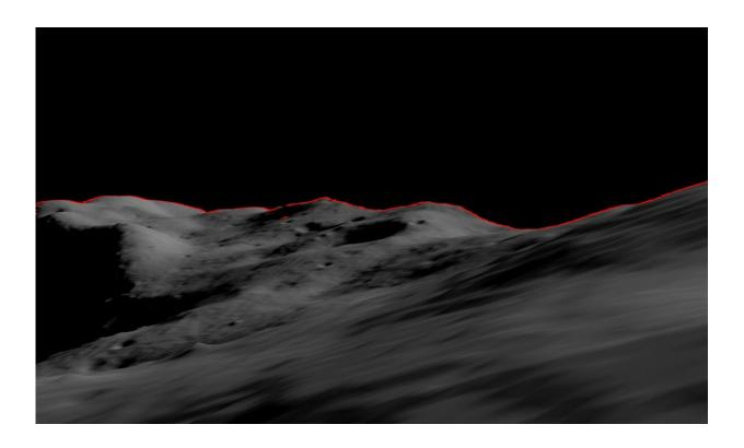
The collection of ridges, craters, and boulders that form a lunar horizon can be used by an artificial intelligence to accurately locate a lunar traveler. A system being developed by Research Engineer Alvin Yew would provide a backup location service for future explorers, robotic or human. Credit: NASA/MoonTrek/Alvin Yew
